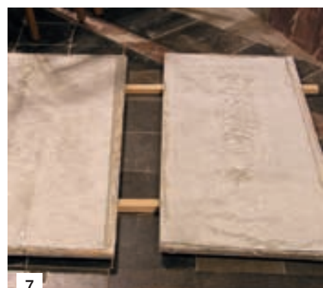
Photo 9. Determination of the deformation behaviour of the sandwich elements in the climate chamber.
