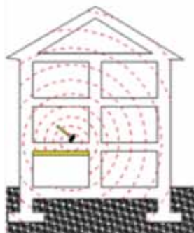
Figure 1. Impact noise is propagated through walls, making the insulating action of false ceilings ineffective.
