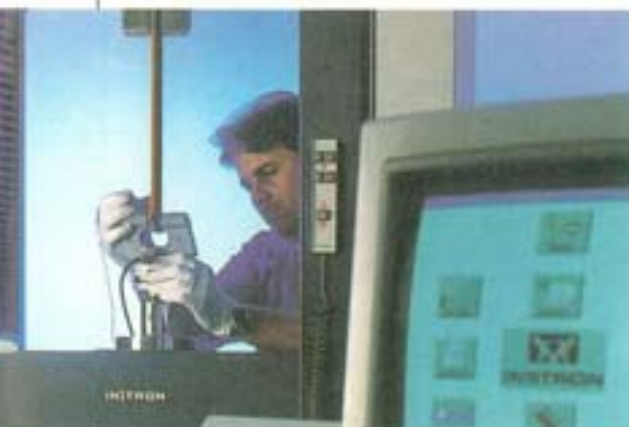
Left, tear resistance test on the MAPELASTIC polymer-cement system using an Instron electron dynamometer.
