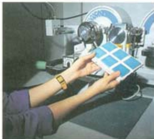
Below, x-rays diffractometer; this equipment determines with extreme precision the chemical composition of materials.
