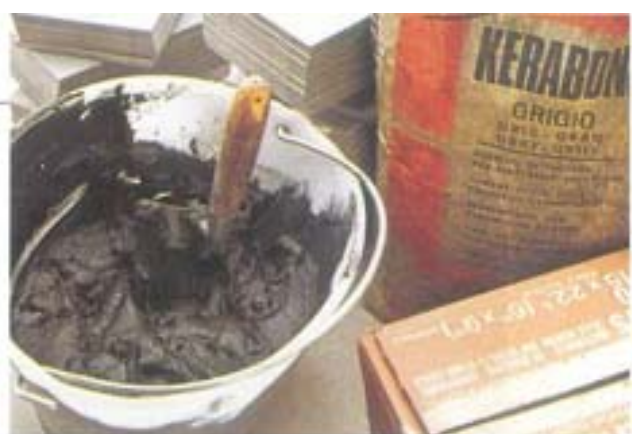
At left, Hewlett-Packard offices, Slezzano, Italy. ADESILEX G19 CONDUCTIVE tests used to install pvc flooring At right: conductive cementitious adhesive used to install conductive ceramic tiles
