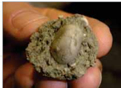
FIGURE 1. Composition of fresh aggregate produced with RE-CON ZERØ
