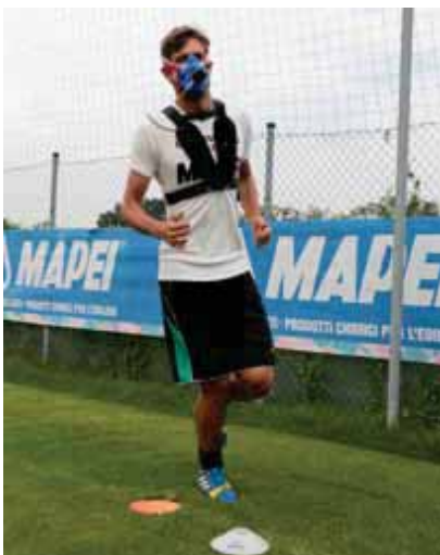
PHOTO 2. A Sassuolo player wearing a metabolic cart device during a running test to determine the energy cost of running.
