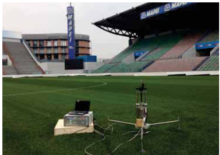
PHOTO 1. The Berlin Athlete test reproduces the stress of an athlete over the tested surface, thus testing the surfaces' mechanical characteristics.
