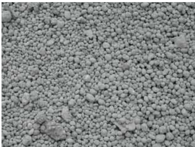
ABOVE. Artificial aggregates made using the HPSS system from soil taken from the former Conterie area.
