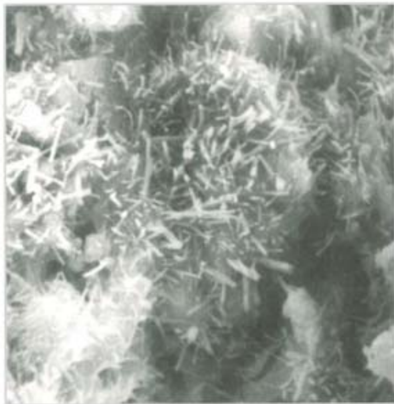
Fig. 4 Microstructure of a cement paste photographed using a scanning electron microscope.
