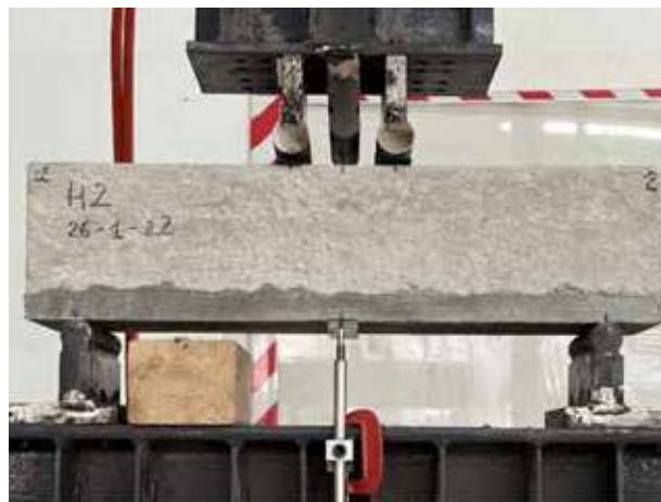
1. Repaired concrete samples subjected to dynamic loads.
