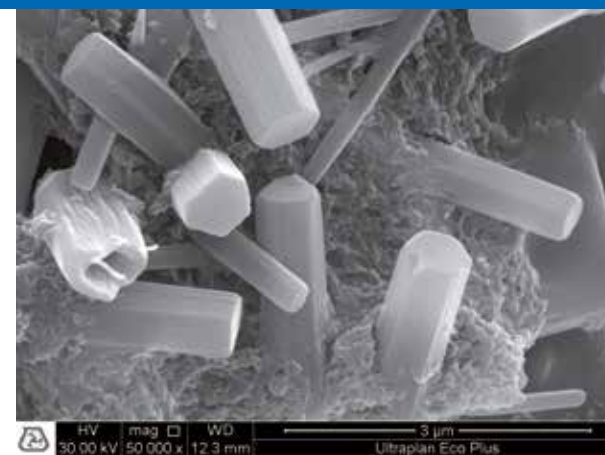
PHOTO 1. Electronic microscope image of ettringite crystals, the chemical species that forms in Mapei binders based on alumina cements. Their features are exploited to obtain rapid products.
