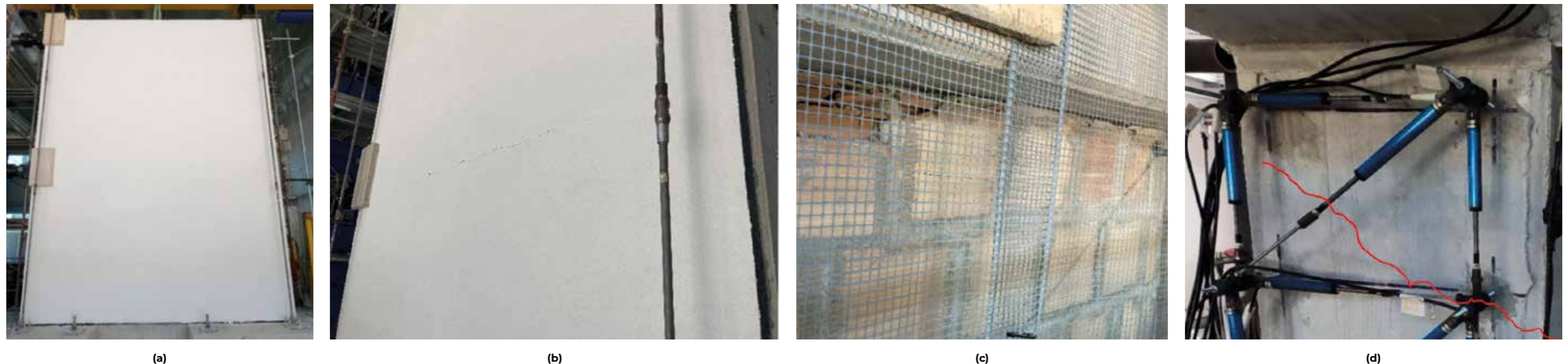
FIGURE 2. Evidence of the damage following testing at 175% of the seismic intensity in L'Aquila in 2009 (PGA = 0.45g): level of damage on the external side (a); damage to the external side with visible horizontal cracks in correspondence with the intrados of the beam at ground-floor level (b); crushing of the first course of bricks at the attachment point with the intrados of the beam at ground-floor level (c); first sign of shear cracks in the lower beam due to the thrust effect of the infill-wall (d).
