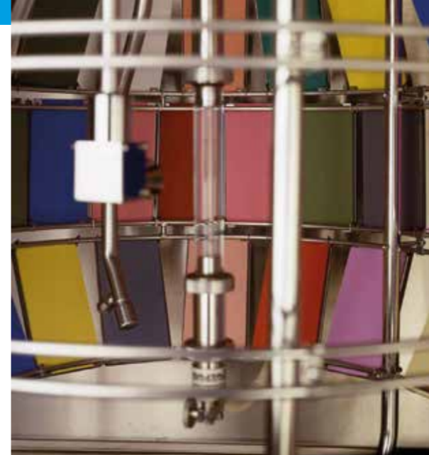
The inside chamber of the Weather-Ometer, the instrument used to simulate accelerated ageing of Mapei products.
