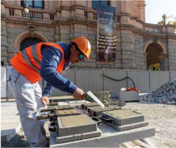
1 and 2. Application and cleaning of MAPESTONE PFS2 FLEX used to grout joints. 3. Samples of the mixes used to install (MAPESTONE TFB 60) and grout (MAPESTONE PFS2 FLEX) the stone paving were tested to make sure they were prepared correctly and complied with the specified performance properties. 4 The completed paving made up of stone slabs and cobblestones and the expansion joint.
