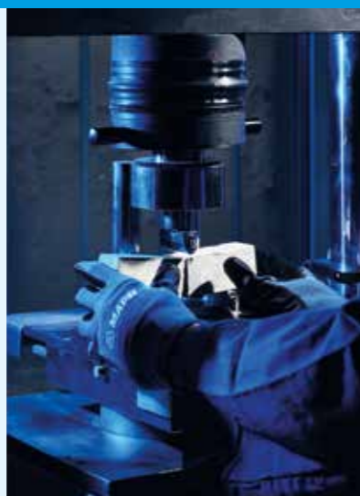
Flexural strength test on a MAPETHERM product according to EN 998-1.
