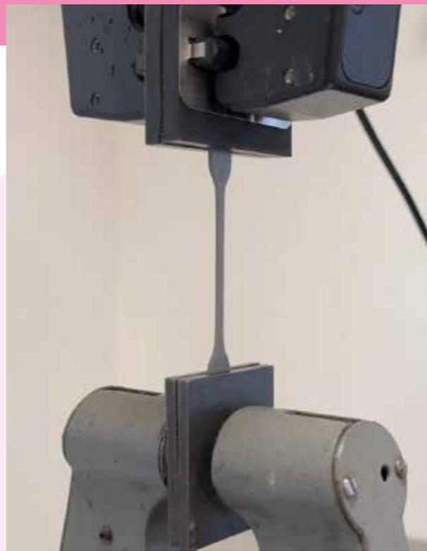
2. Measuring the mechanical characteristics of polyurea.
