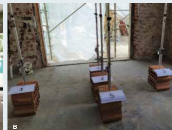
Fig. 2. Area of load test and measuring instruments at ground level in a) pre-strengthening phase b) post-strengthening phase.
