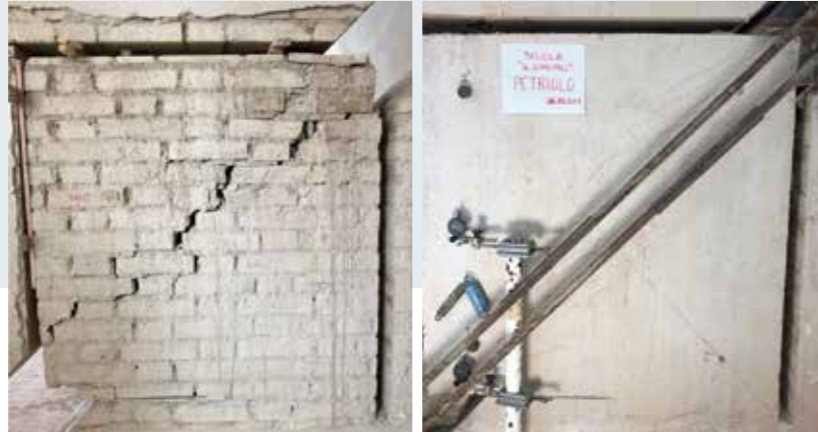
Comparison of the failure mode of a panel without strengthening (left) and strengthened with PLANITOP INTONACO ARMATO (right).
