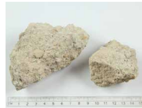
Samples of mortar taken from the existing masonry were analysed in the Mapei R&D Laboratories to examine the grain size, the soluble salts content and the mineralogical composition.
