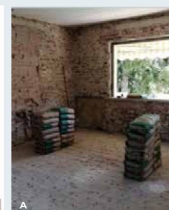
Fig. 3. Area of load test and measuring instruments at first floor in a) pre-strengthening phase b) post-strengthening phase.
